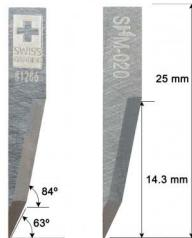
**Description:** Long-Life oscillating knife. Similar to HTZ-020 (Z20) but with better performance. Very fine, delicate knife with minimal overcut; designed for cutting complex geometries, small radii and complex details.
