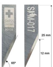
**Description:** Long-Life oscillating knife. The overcut is smaller, but the knife exerts more drag force on the material than the SHM-016. For best results, use as an oscillating knife.
