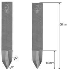
**Description:** Double-sided Knife for less tough, fibrous materials. This knife offers similar properties to Z11 (HTZ-013 and the HTZ-045).
