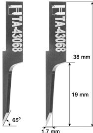
**Description:** Identical knife to the HTZ-028 but with smaller turning radius (2 mm.).
